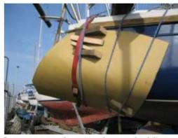
[View from stern showing baton holding mould in place before filleting and gelcoat]
