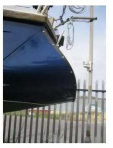
BOLT MATERIAL: I used stainless 10mm A4 and A2 nuts and bolts and washers, with the A4 (marine resistant) bolts on the Sugar scoop stern extension pointing in. The reason to use different grades was explained to me by Debbie at Margnor Fastenings near Guildford (great for stainless fastenings at normal prices). That if you use the same grade stainless it can 'Gall' or pressure weld when fully tightened.
