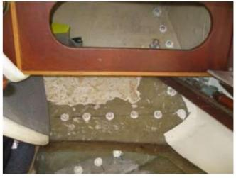
INSIDE: I was going to have to be able to reach the whole stern bulkhead which entailed peeling back some carpet which was the existing lining and cutting out some of the rear seat panels. All carpet was later replaced when I re-lined the boat with vinyl.
