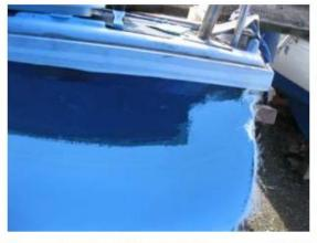
I used pigmented gelcoat and applied two layers so I had enough thickness to rub out any slight imperfections. I was fortunate to have Oxford Blue pigment that is the same colour as the hull (though I did paint the extension so it was a perfect match). I also partially covered the stern of the boat and used a fan heater to warm it up before applying the gelcoat as the weather was cool.
