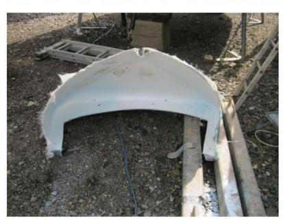
lower fastening bolts in place with a slight downward angle. Just enough to shed water. This meant that I would have to fit a good quality hatch later to access the fixings. At this point I painted a layer of waxed gelcoat (flowcoat) over the inner surface to get a smooth impervious finish.
