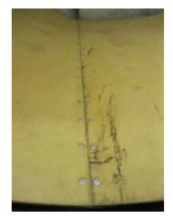
I then waxed both sides thoroughly, inside for release from the gelcoat and outside for weather protection (I was doing this in the boatyard and the only protection was a tarpaulin).
